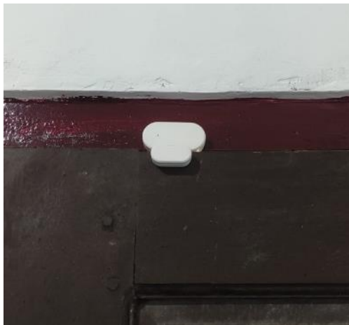
Figure 8: Door Sensor on the Door of the Software Laboratory Room
