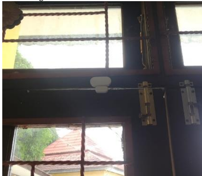
Figure 2: Door Sensor Device at the Entrance of Dormitory 1
