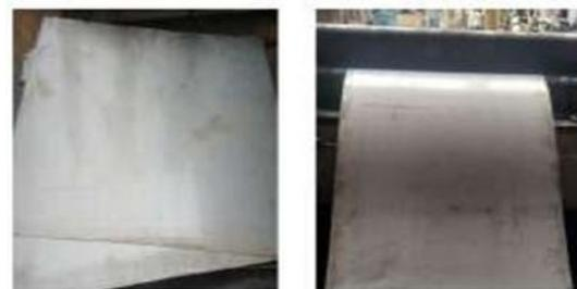
Gambar 2.3 (a) Plat Stainless Steel /SS 201 tebal 2 mm, (b) Plat SS 201 di roll
